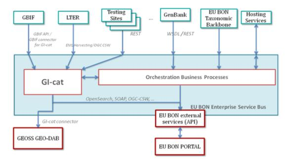
Figure 2. Proposed architecture for EU BON consisting of a hybrid solution in which GI-cat in integrated in the enterprise service bus.
