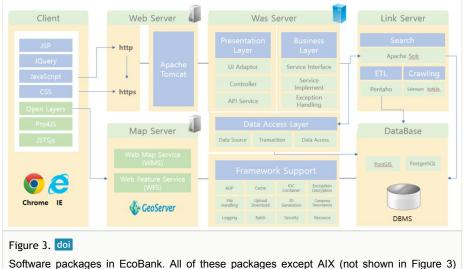
Software packages in EcoBank. All of these packages except AIX (not shown in Figure 3 used in the system architecture of EcoBank, are open-source software.
